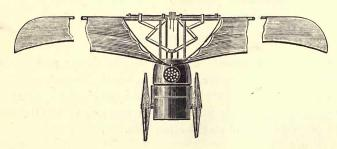
carriage, and these wings are flapped up and down by the action of a steam-cylinder.
